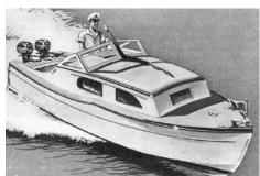
Dolphin A 16 ft boat specially designed for those who move their craft about by trailer. The hull is light enough to be transported anywhere by trailer and the boat is of a size to be easily handled. It will accommodate two persons for extended trips or a party of 4 for day cruises and do it comfortably.
